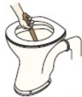
Unblocking a toilet
